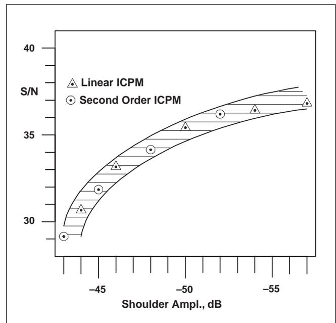
Figure 12. Shoulder amplitude vs s/n caused by phase error.
