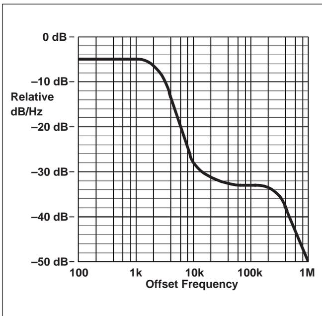
Figure 13. Phase noise spectral model.
