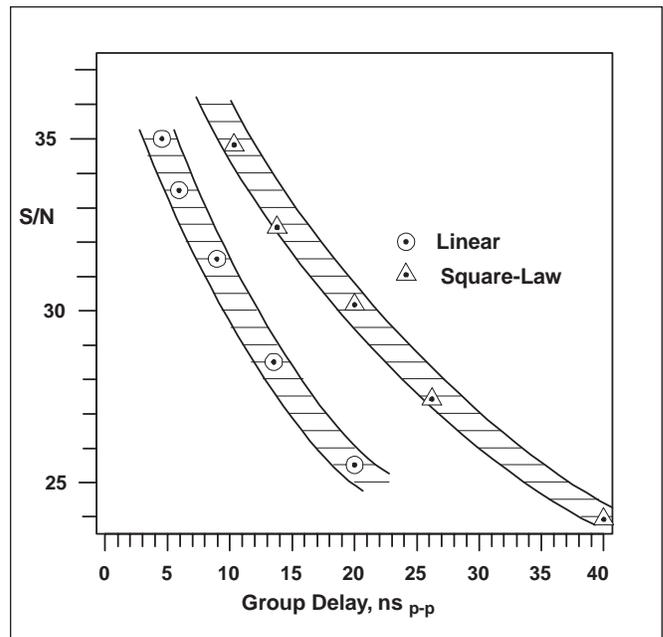
Figure 7. Measured S/N as a function of group-delay error.
