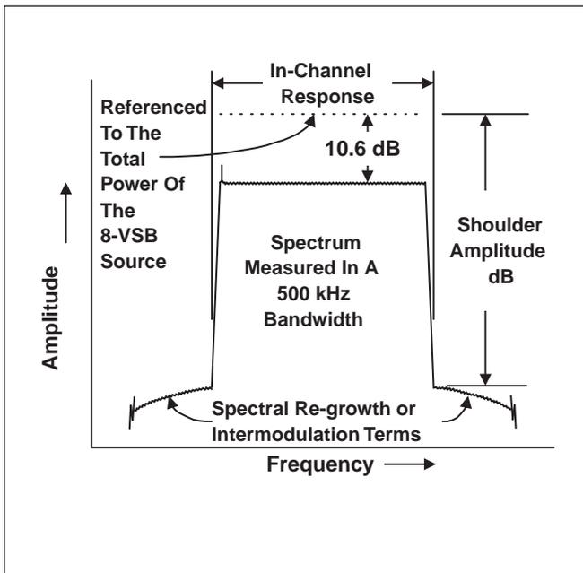
Figure 16. Spectral content of DTV transmission showing definition of shoulder amplitude.
