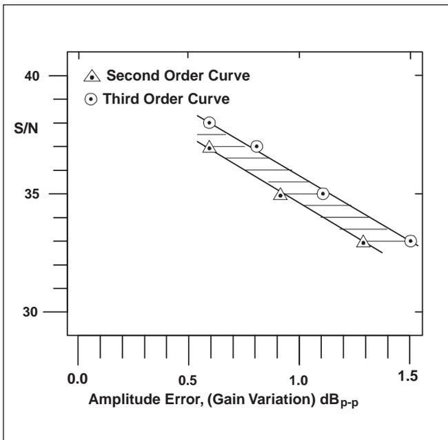
Figure 9. S/N impairment caused by amplitude error.
