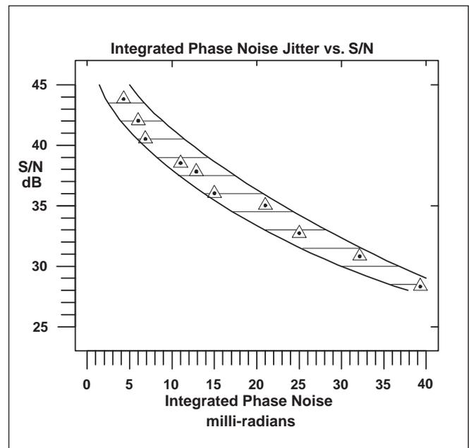
Figure 14. S/N as a function of integrated phase jitter.
