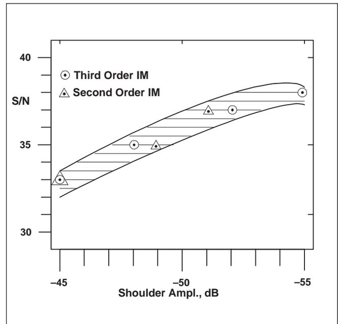
Figure 10. Shoulder amplitude caused by amplitude error.
