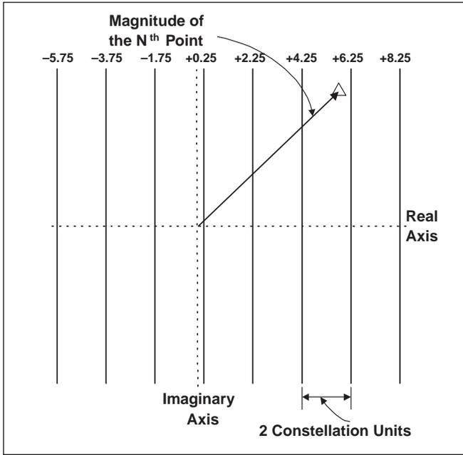
Figure 15. 8-VSB constellation with illustration of Signal magnitude.
