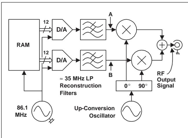
Figure 2. Simplified block diagram of precision 8-VSB source.
