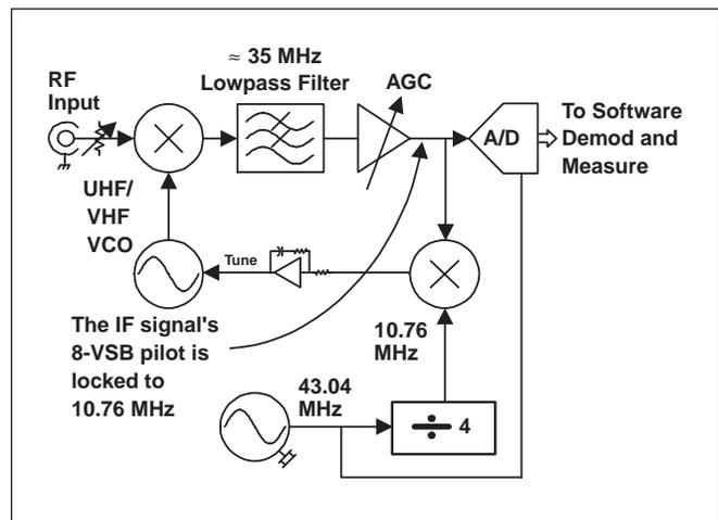
Figure 3. Very simplified block diagram of a 8-VSB measurement test set.
