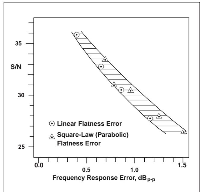
Figure 5. Measured S/N vs Frequency Response Error.
