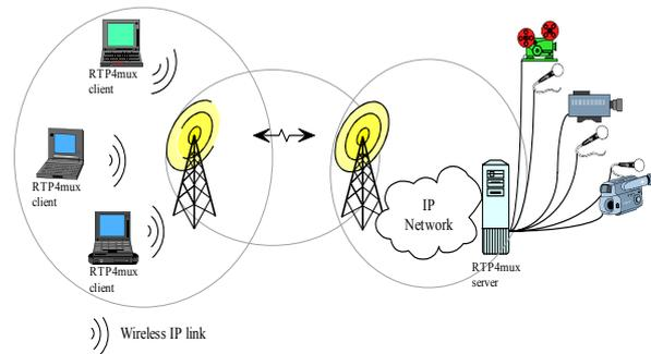
Figure 6: Videoconferencing over wireless IP network using RTP4mux Gateway.
