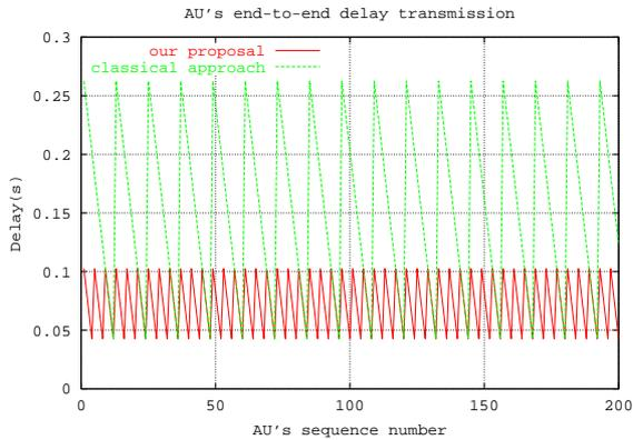
Figure 10: End-to-End AU's transmission delays, calculated between the coding generation time and the decoder reception Time.
