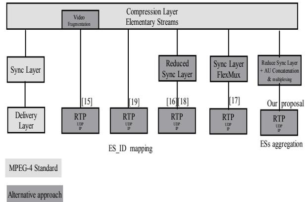
Figure 2: Concurrent approaches for encapsulating MPEG-4 streams over IP.
