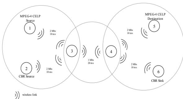
Figure 9: The wireless IP network Model.
