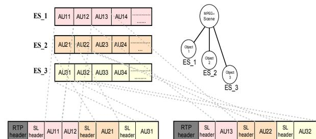
Figure 3: Elementary Streams encapsulation process.
