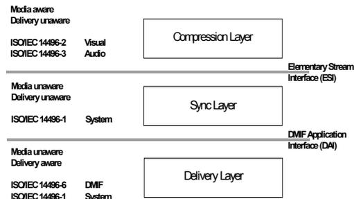
Figure 1: MPEG-4 System Architecture.
