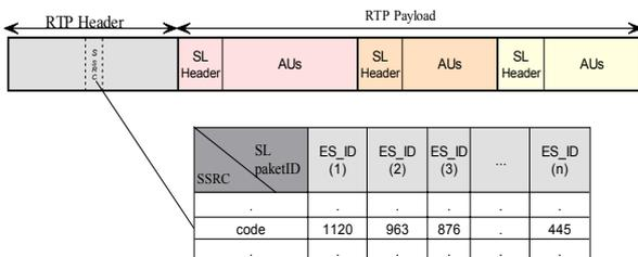
Figure 4: ES\_IDs signaling through the RTP header.
