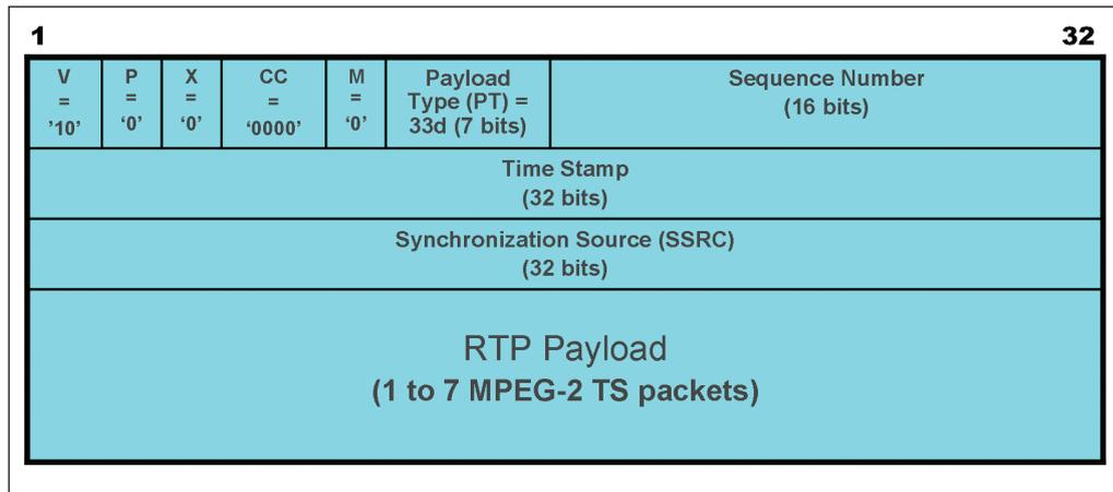
Figure 1. RTP format for encapsulating MPEG-2 Transport Stream within IP packets. V = Version, P = Padding, X = eXtension, CC = Contribution source count, M = Marker, PT = Payload Type.
