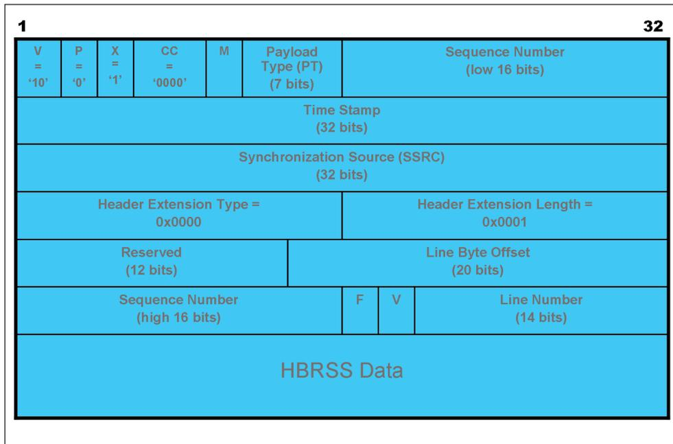
Figure 2. RTP format for encapsulating HBRSS within IP packets. V = Version, P = Padding, X = eXtension, CC = Contribution source count, M = Marker, PT = Payload Type.
