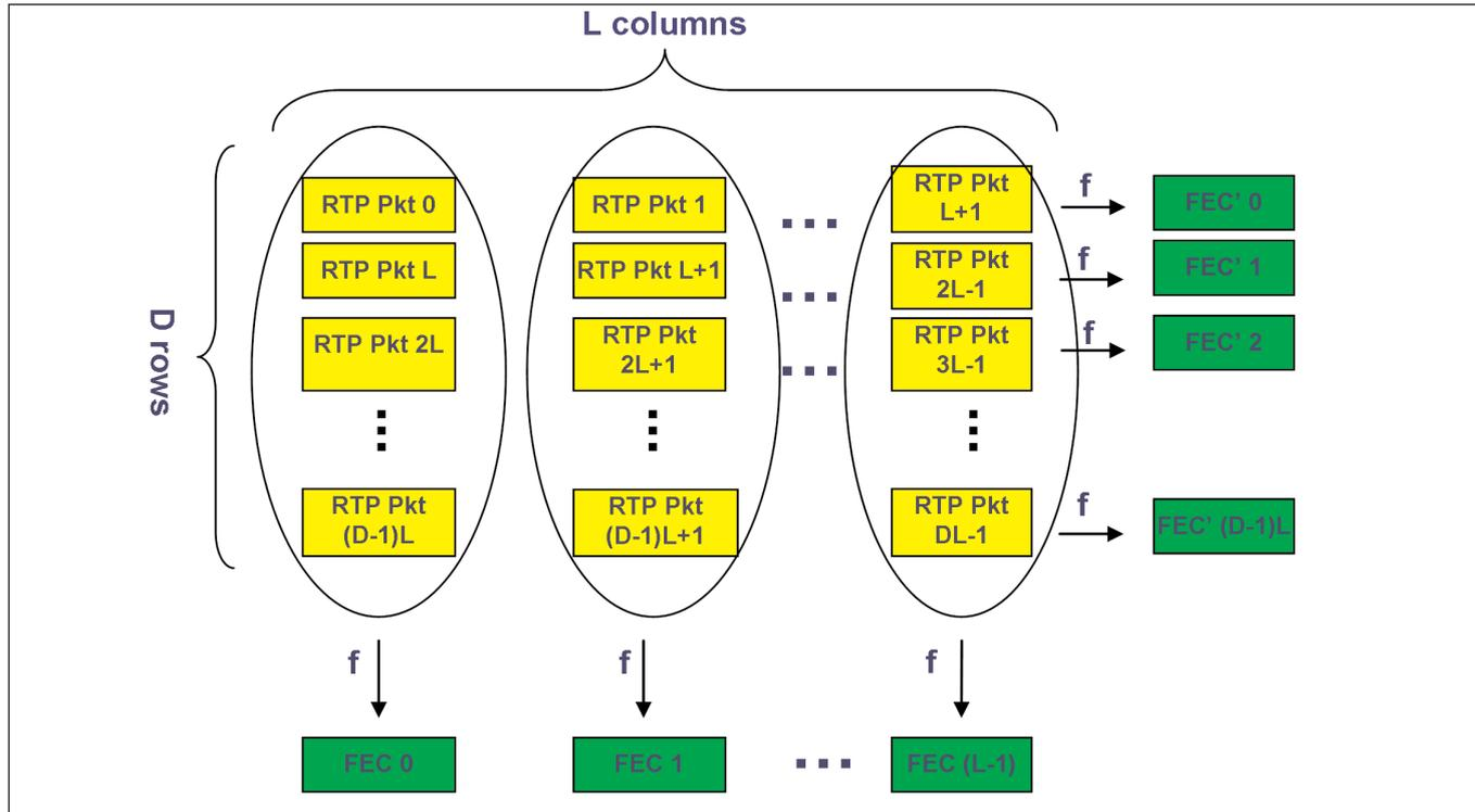
Figure 3. Example of matrix structure for FEC computation.
