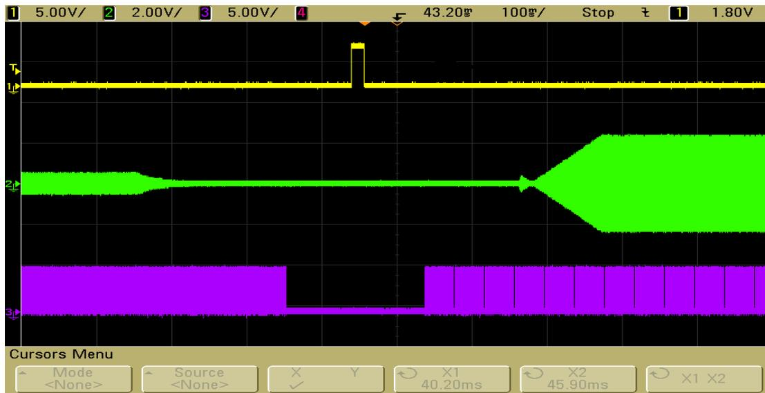
This shows the PCM being faded down as normal, followed by the section of silence. Normally the Preset would be the predominant signal, but as the mixer knows it is DE, it inserts silence until the fade has reached full amplitude before cutting up the DE signal. (Followed by the two-frame recovery by the decoder).
