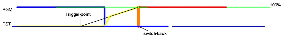
The advantage of this process is the short time delay involved, which minimises lip-sync issues. The audio delay is a mere 8 samples (plus any delay needed to align two Dolby E packets). This compares to the alternative of a full frame of delay in a Dolby decoder, and another full frame in an encoder.
