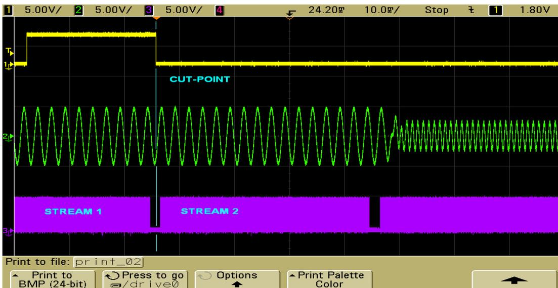
The falling edge of yellow trace indicates where the Program co-efficient reaches zero & *the end of packet has passed*. The purple shows the decoded AES containing Dolby-E data out of the mixer, the gaps being the guard bands, in sync with the Vertical interval of the video reference used to time the system.
