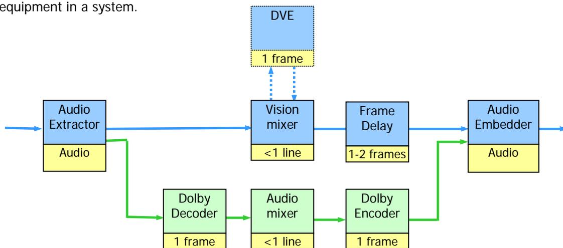
Clearly the video and audio path can have a significant difference in delay, up to 2 frames if a DVE is not present, and one frame if the DVE is present. This causes serious lip-sync issues. The solution would normally be to insert a frame delay into the video path as shown, incurring additional expense and using valuable rack space.
