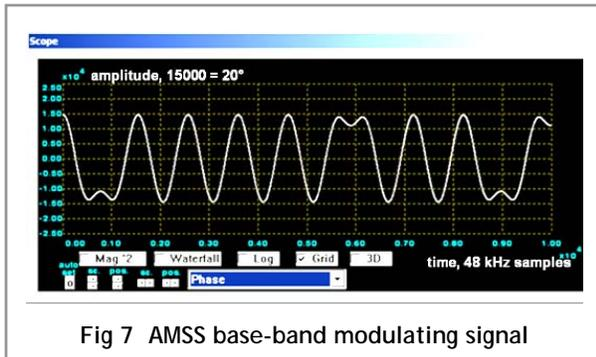
Fig 7 AMSS base-band modulating signal
