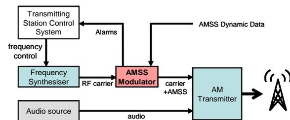
Fig 4 AMSS Modulator interface with Tx
