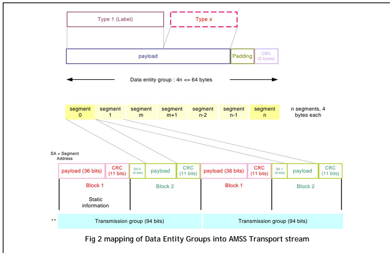
Fig 2 mapping of Data Entity Groups into AMSS Transport stream
