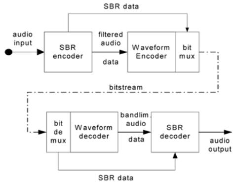
Figure 3: SBR acts as a pre-process at the encoder side, and post-process at the decoder side.
