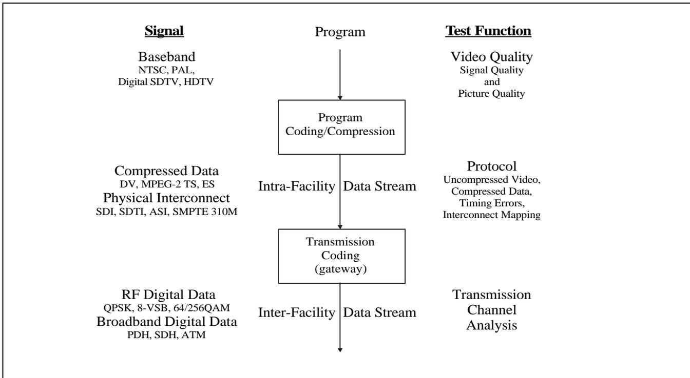
Figure 2. Digital television testing layers.
