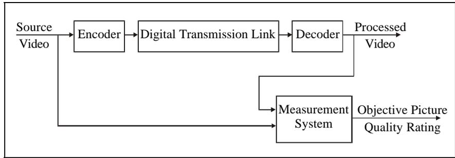
Figure 3. Picture comparison test method.
