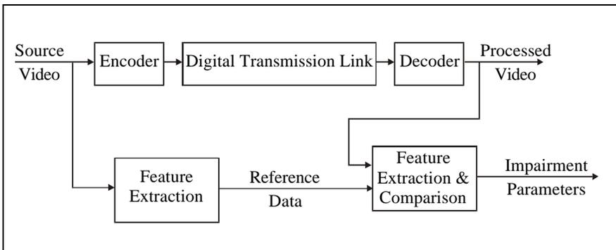
Figure 5. Feature extraction test method.
