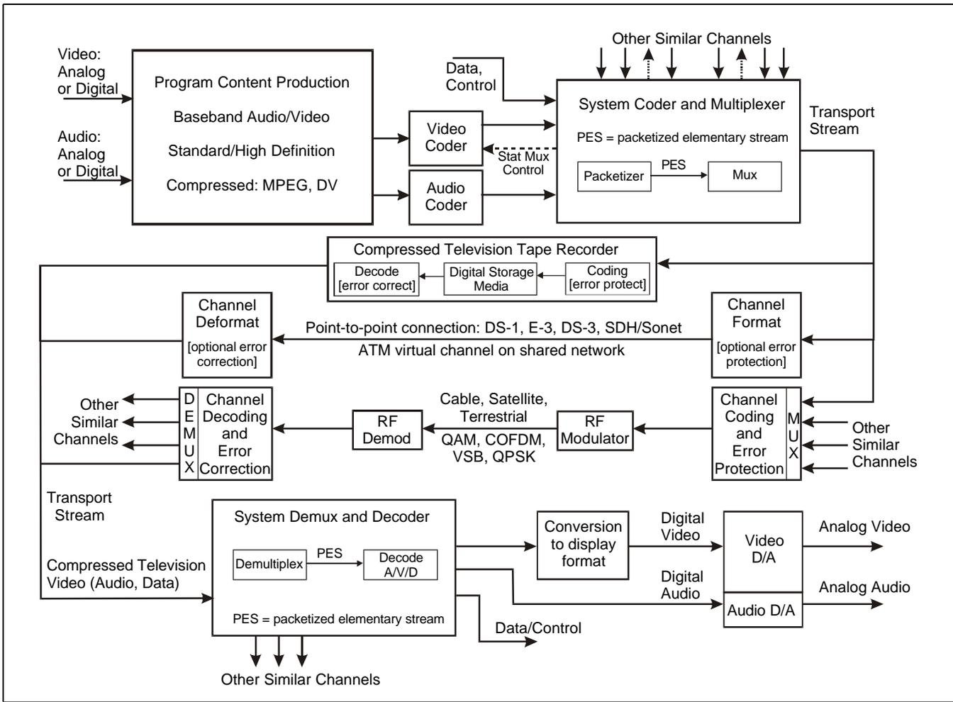
Figure 1. Digital television simplified block diagram.
