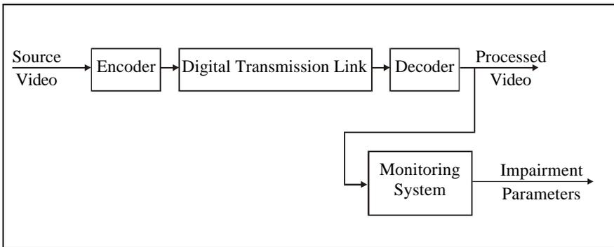
Figure 6. Single-ended test method.
