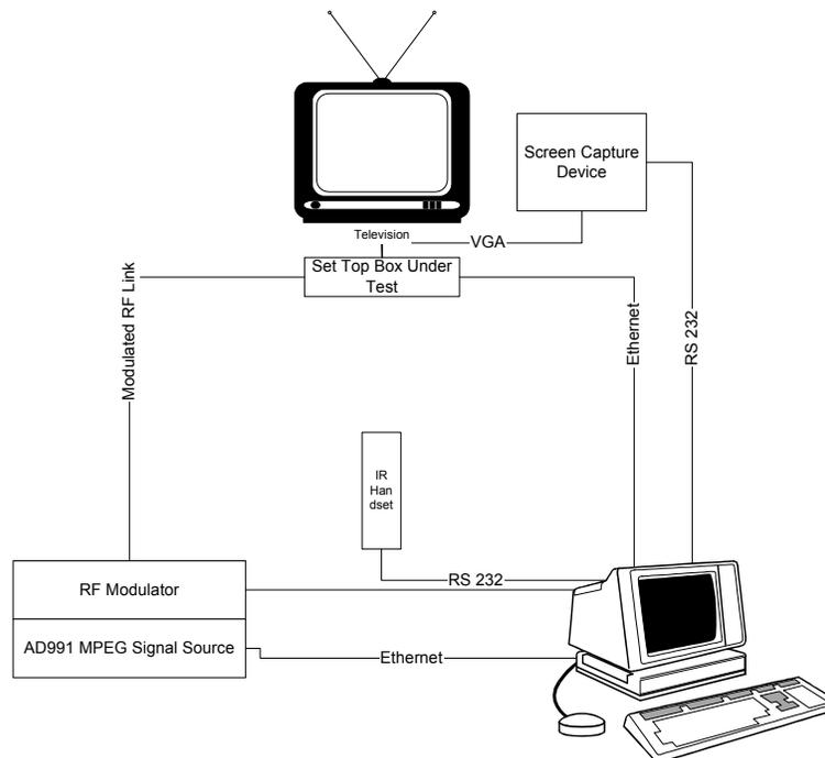
Figure 7 - Automated MHP Set Top Box Verification
