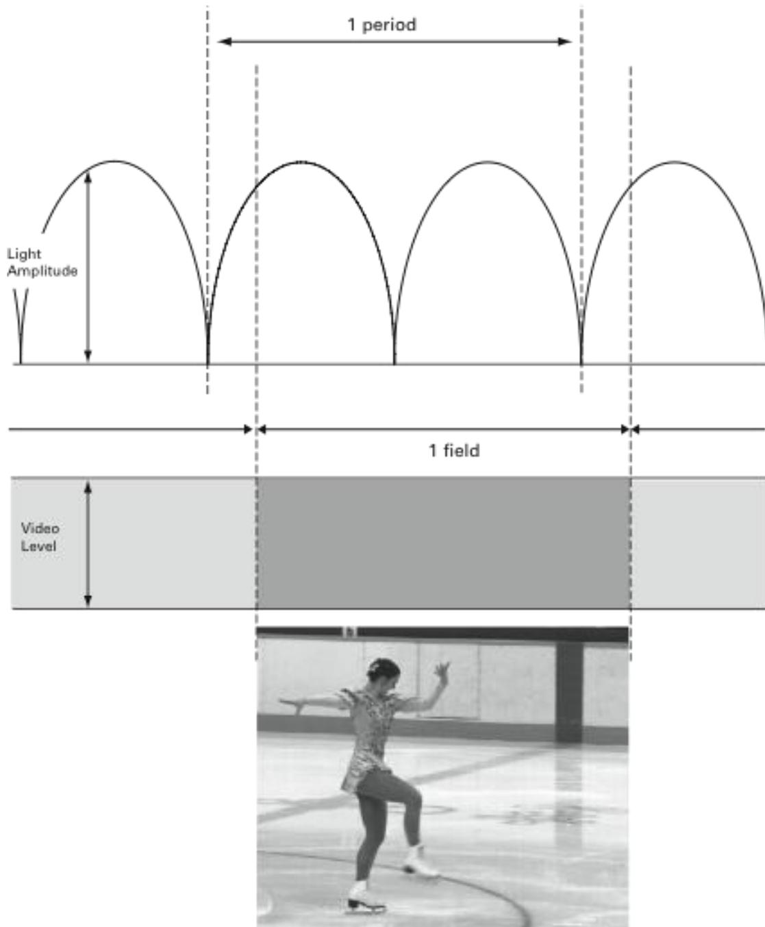
But when shooting at 150 or 180 frames per second, successive frames will receive a different amount of light because each will capture a different part of the power sine wave. When slowed down, these changes in light levels will appear as a visible and distracting flicker.
