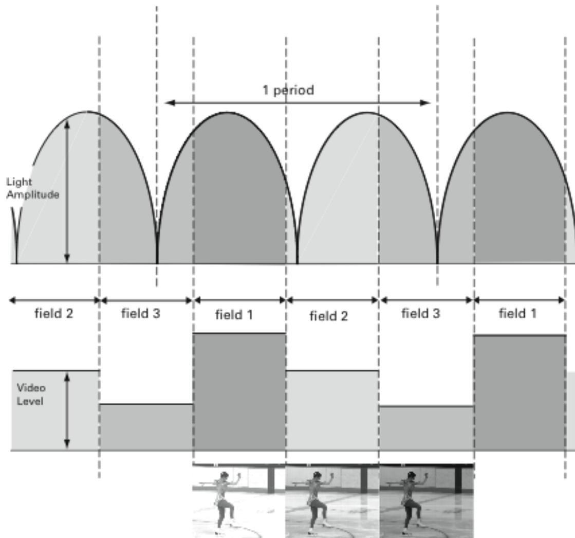
This flicker appears not just with single-phase lighting but also with two- or three-phase lights and discharge lamps.
